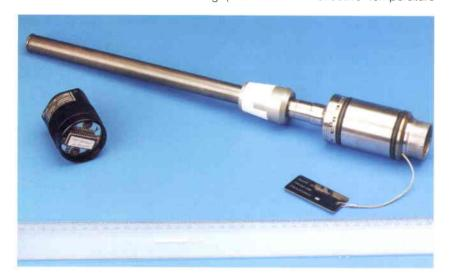
Figure 8. Typical furnace cartridge (AGHF facility)
